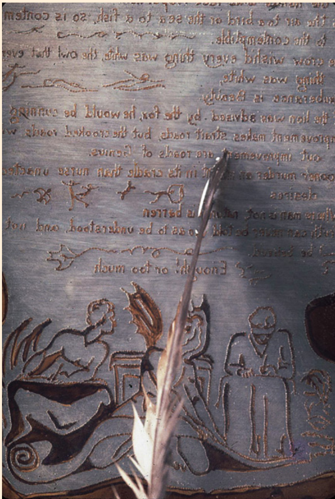
6. Facsimile of Marriage plate 10 as relief etching: biting the plate in nitric acid and feathering the gas bubbles away from the design.
